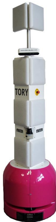
Fig. 1: Autonomous inventory taking robot TORY for RFID-tagged items (MetraLabs GmbH, Germany, 2019).
