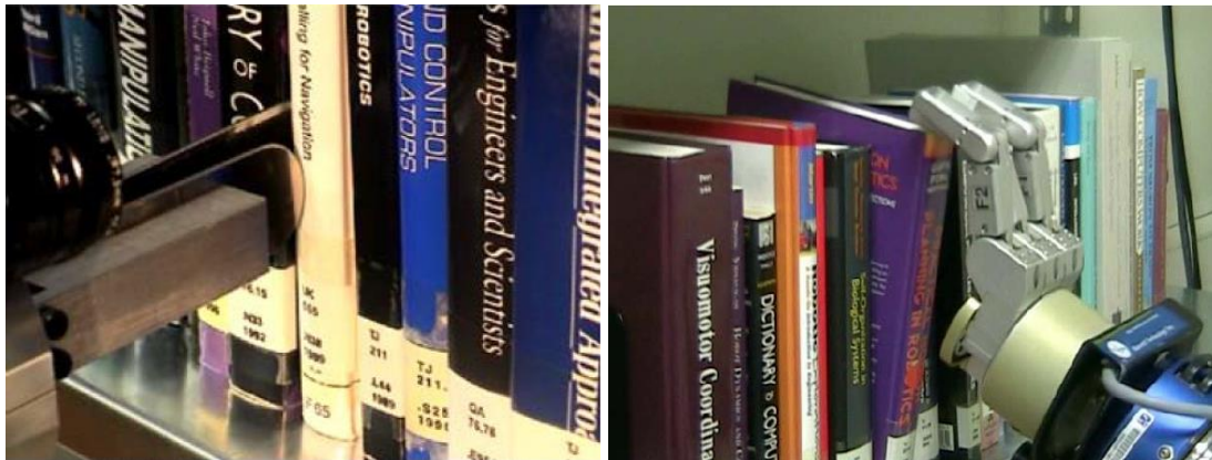
Figure 1. Book grasping based on the considered robotic gripper: parallel jaw (left) and Barrett hand (right)
